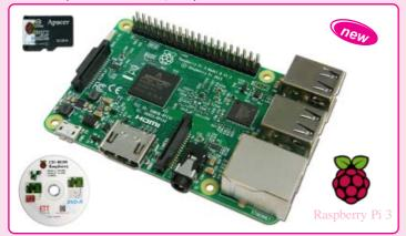
• CPU uses BROADCOM BCM2837 64 BIT QUAD CORE 1.2GHz that is more speed than the old PI model approx. 50-60%, RAM 1 GB
