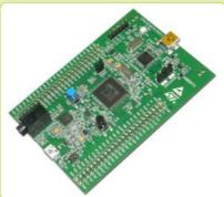
This STM32F407G-DISC1 is designed by ST to replace STM32F4 DISCOVERY; all specifications are the same. There are 2 parts on Board; DOWNLOAD, DEBUG, and MCU.
