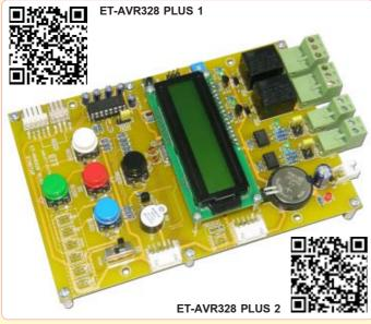
This semi-finished Board Microcontroller uses CPU AVR No.ATMEGA328; write program C Language of Arduino. Write and DOWNLOAD program simultaneously to CPU directly through PORT RS232. There is LCD Display, 2-CH OUTPUT RELAY, 2-CH INPUT DC, RTC with BAT 3V, RS232 PORT, 5 KEY, and others on board. SPECIFICATIONS of ET-AVR328 PLUS 1 and ET-AVR328 PLUS 2
