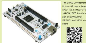
A part of ON BOARD DOWNLOAD and DEBUG is ST-LINK V2-1 to DOWNLOAD Program and DEBUG the operation through PORT USB MINI-B; moreover, it provides Connector SWD to connect DOWNLOAD DUBUG outside Board NUCLEO conveniently.
